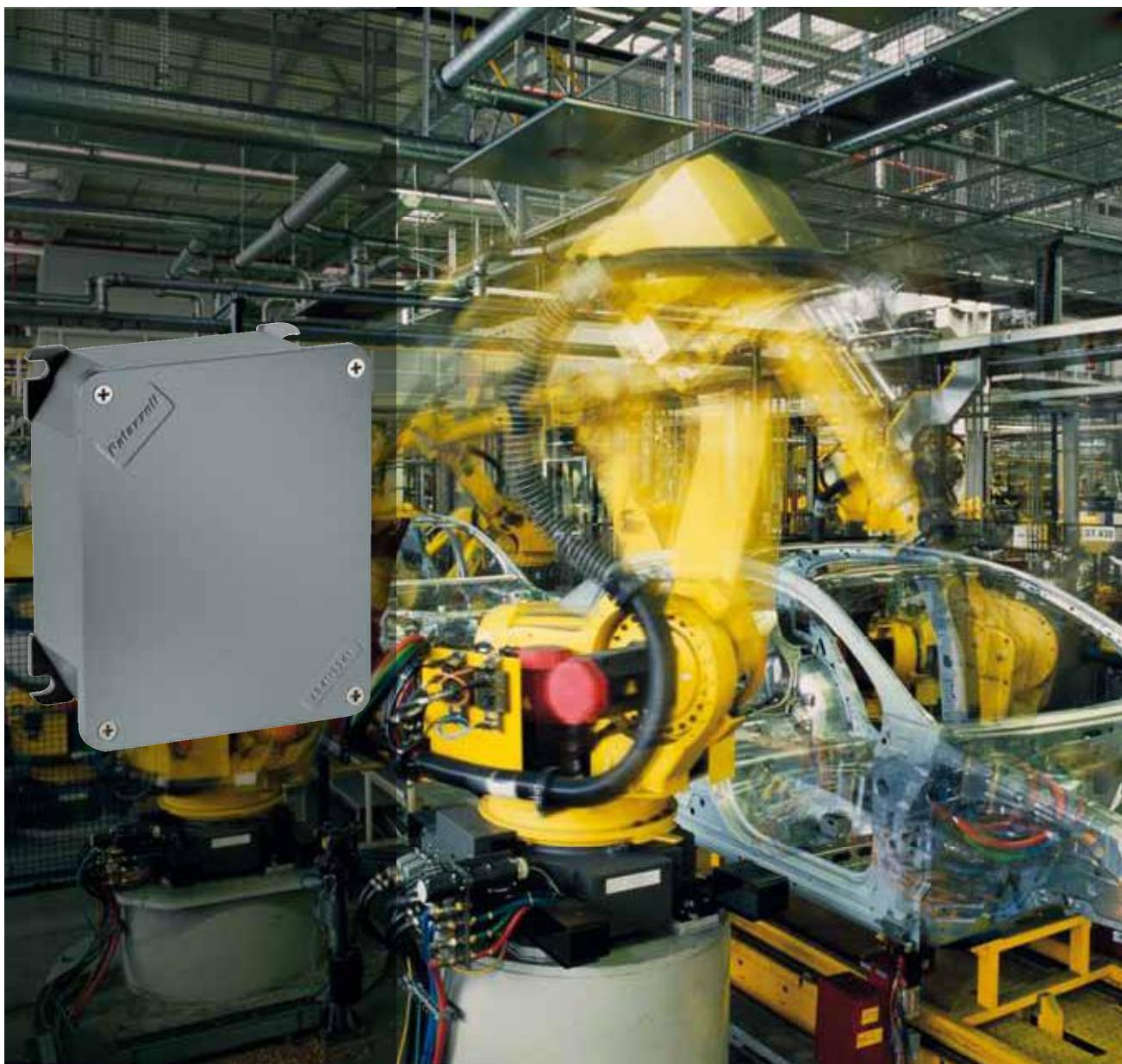
UNiversal BOXes in aluminium alloy are suitable for environments with aggressive atmosphere present. Back box and cover are treated with ecological anticorrosion passivation with fluoro-zirconium and finished with hot polymerized scratch-resistant non-toxic polyester painting.
